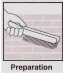
Surfaces must be clean and free from contamination. Loose spalled and eroded concrete should be removed. Thorough cleaning and roughening of any surface to which the product is being applied is absolutely essential for a successful repair. Prepared surfaces should always be primed with Superquartz L.W. primer. The mixed primer should be applied immediately using a stiff bristle brush, working the material into the prepared surface to obtain maximum penetration.
