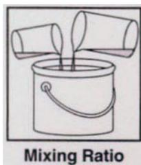
Superquartz L.W. 2 parts to 1 part activator by weight. Thoroughly mix the resins together to form a uniform material. Add the aggregate immediately until a desired consistency is achieved. The complete material should then be mixed thoroughly for 2-3mins to produce a uniform material. Prolonged hand or mechanical mixing will provide a wetter mix. Primer: 2 parts base to 1 part activator by weight.
