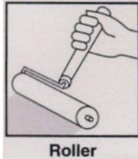
An even consistency is quickly obtained and the resultant creamy compound is simply poured onto the previously primed surface generally spread about with a trowel or squeegee then rolled out using a spiked roller. Use thin laths or foam draught excluder to retain the mixture within the area to be treated.
