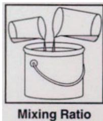
AWF Glazecoat/Machine Guard is a two part material consisting of a base and activator resin. The base should be poured into a suitable mixing container and stirred for 2-3 minutes. The activator should be stirred for 2-3 minutes then added to the base resin and stirred for at least 5 minutes or until a homogenous mix is obtained.
