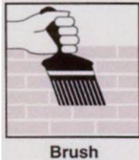
Application should not be carried out at temperatures below 5°C nor when relative humidity exceeds 85% or when the surface to be coated is less than 3°C above the dew point.
