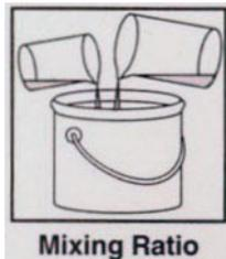
4 parts base to 1 part activator by volume. The base component should be thoroughly stirred to incorporate any slight separation, whilst continuing stirring, the contents of the activator should be added. Continue stirring for at least 5 minutes until a homogenous mix is obtained. Failure to do this will result in an extended cure time. Following mixing, stand for a further 5 minutes.
