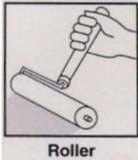
Roller application should be carried out with a short haired lambs wool roller ensuring that the material is spread over the surface evenly.
