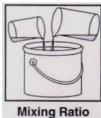
AWF Floortect XSL is a three component system consisting of a Base, Activator & Aggregate. Mix the base resin and activator separately and then mix well together. After mixing, continue stirring and add the total contents of the aggregate. The use of a mechanical mixer would be advantageous.
