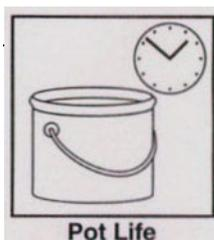
Once you have mixed the Base, Activator and Aggregate together, you have approximately 20 mins to use the mixed material.
