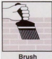
Surfaces which are porous should be primed with AWF S.P.Primer. AWF HBD should be applied by Brush or roller. Re-coating should take place as soon As possible to achieve good intercoat adhesion Properties, preferably on the following day. If more Than one day elapses between coats, abrade the Surface lightly (with glass paper) before re-coating. Two coats are recommended for long term protection. All equipment must be cleaned immediately after use With AWF Universal cleaner.
