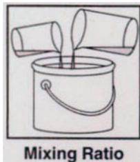
Floortect H.B. is a two part material consisting of a Base & Activator resin. The base and activator should be mixed separately for 2-3 minutes before being mixed together for 4-5 minutes until a homogenous mix is obtained.
