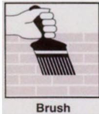
Apply Flexseal Aluminium to the prepared, dry surface using a soft bristle broom and spread at the rate of 0.75 litres per sq.m. When product is dry, apply a second coat (at the same coverage rate) and if possible, apply at right angles to the direction of the first coat. This will ensure complete and uniform coverage.
