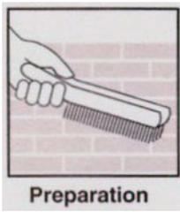
All existing dirt, oil and grease should be removed and the surface wiped with AWF Universal Cleaner. Any areas of frayed or fragmented rubber should be cut away to provide a sound repair area. Smooth surface including metals should be mechanically etched to produce a good preparation profile with abrasive blasting being preferred for metal substrates. Rubber surfaces are best roughened using a stiff wire brush. Edges of repair areas of belts, hoses, tyres etc should be undercut.
