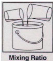
AWF Flexible Rubber 60 F.G. is a two part material consisting of a Base & Activator resin which must be mixed together prior to use. The Base should be poured into a suitable mixing container and stirred thoroughly. The Activator should be added to the Base Resin and thoroughly mixed together to produce a streak free viscous liquid. Thorough mixing is extremely important and once the material appears mixed a further period of mixing should be carried out to ensure there is no unmixed material.
