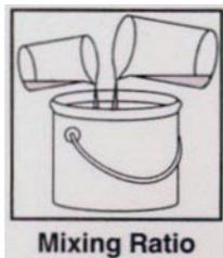
AWF E.M. Rapid 10 is a two part material consisting of a Base & Activator resin which must be mixed together prior to use. Mix 1 part Base to 1 part activator onto a clean board or other suitable surface. The two resins should then be mixed thoroughly together to produce a completely streak free material. The mixed material should be used within 3 minutes of mixing at 20°C. This time will be reduced at higher temperatures and extended at lower temperatures.
