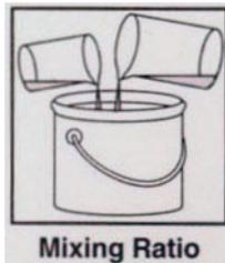
AWF E.M. Liquid Ceramic-Flex F.G. is a two part solvent free material comprising Base & Activator components which must be mixed together prior to use. Add all the contents of the activator container into the base container and mix thoroughly. Alternatively measure three volumes of base and one volume of activator into a clean container and mix until completely streak free.
