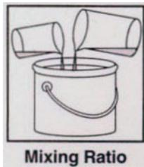
AWF E.M. Liquid Ceramic-Flex E.G. is a two part solvent free material comprising Base & Activator components which must be mixed together prior to use. Add all the contents of the activator container into the base container and mix thoroughly. Alternatively measure three volumes of base and one volume of activator into a clean container and mix thoroughly.
