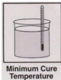
This product should not be used if the temperature or the surface to be coated falls below 5°C.
