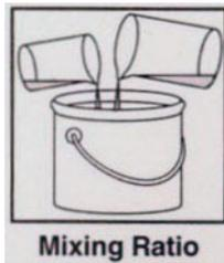
AWF E.M. Ceramic Metal E.G. is a two part material consisting of a Base & Activator resin which must be mixed together prior to use. Measure three volumes of the Base resin and one volume of the activator resin onto a clean mixing surface. The two resins should be thoroughly mixed together until completely streak free.
