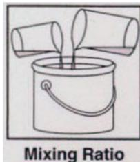
Chemi-TECT S.C. is a two part material consisting of a Base and Activator resin. The base should be poured into a suitable container and stirred for 2-3 mins. The activator should be stirred for 2-3 mins then added to the base resin and stirred for at least 4-5 mins or until a homogenous mix is obtained.
