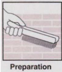
Steel Surfaces: For immersion conditions should be abrasive blast cleaned to a minimum SA21/2 BS7079 Part 1 1989 or equivalent. For other applications, particularly where blast cleaning is not practical, manual wire brush or grinder should be carried out.
