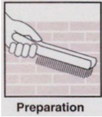
Drill the required number of holes allowing 2mm extra diameter above fixing size (for depth see coverage chart) Remove all dust from the hole, before injecting A.W.F. Anchor-Set/Mini Anchor-Set ensuring the holes are dry, clean and sound. If using as an adhesive, ensure surfaces are clean, sound and free from contamination.
