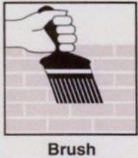
Apply by brush or mop. Metal components can be soaked in a tank. To ensure thorough cleansing of components, agitate if necessary until any effervescence ceases. Finally, rinse down the treated area/components thoroughly with water.
