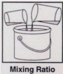
Can be used directly as supplied from the container. For a less concentrated solution, Acid Etch can be diluted with up to 8 parts warm or cold water. When diluting the product, always add Acid Etch to water, never water to Acid Etch.
