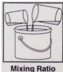
Stir the contents of the base and add the entire contents of the activator. Stir for a full 5 minutes using a slow speed drill (400 – 500 rpm) with a mixer paddle until a completely homogenous mix is obtained. Take care to avoid including excess air. Mixing is made easier if the activator is added and mixed in two stages. Pour immediately into the primed joint.
