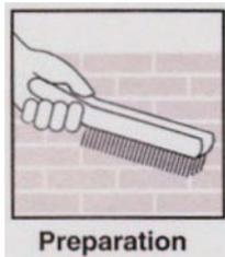
The joint must be completely dry and free from all traces of dirt, dust, grease and previous sealants. etc. Cleaning can be carried out by mechanical wire brush, angle grinding, sand/grit blasting. All joints should then be blown out clean, dry, oil free compressed air to remove loose matter. In all cases, a clean bonding surface must be obtained.
