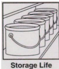
Indefinite when stored in original sealed containers between 5°C (40°F) and 40°C (104°F) in dry conditions.
