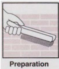
All existing dirt, oil and grease should be removed and the surface wiped with AWF Universal Cleaner. Any areas of frayed or fragmented rubber should be cut away to provide a sound repair area. Smooth surfaces including metals should be mechanically etched to produce a good profile with abrasive blasting being preferred for metal substrates. Rubber surfaces are best roughened using a stiff wire brush. Edges of repair areas of belts, hoses, tyres etc should be undercut.
