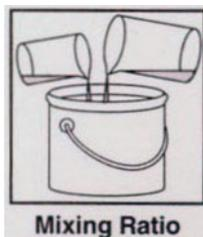
AWF Flexible Rubber 60 E.G. is a two part material consisting of a Base & Activator resin which must be mixed together prior to use. Two volumes of the Base and 1 volume of the Activator should be measured onto a clean surface and the two resins mixed thoroughly together to produce a smooth streak free material. Thorough mixing is extremely important and once the material appears mixed, a further period of mixing should be carried out to ensure there is no unmixed material.
