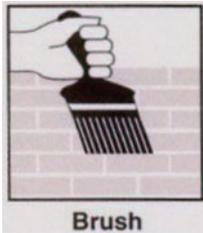
AWF Clearshield should be applied liberally to the prepared surface using pneumatic spray or a large paint brush. Application should start at the highest point of the surface to be treated allowing excess material to drain down the surface. One coat is sufficient for most surfaces, however on very porous surfaces a second coat should be applied as soon as the first coat is dry. All equipment should be cleaned immediately after use with AWF Universal Cleaner.
