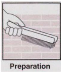
All surfaces should be clean, dry and free from contamination. Any adjacent painted areas such as door and window frames should be protected against contact as AWF Clearshield may cause softening of the paint.
